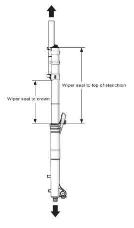
Original distance between wiper seal and top of stanchion:
