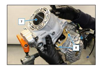
Screw without tightening the nuts (9) then tighten crosswise with a torque of 26 - 28 Nm (2,6 - 2,8 Kgm, 19,18 - 20,65 ft/lb).
