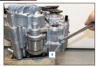
Wait for the oil to drain completely through the hole, clean the sealing surfaces, replace the aluminium washers (2 and 4), remove any magnetic debris (5) of the drain cap (3) and screw the cap back on, tightening to 20 Nm (2 kgm, 14,75 ft/lb).
