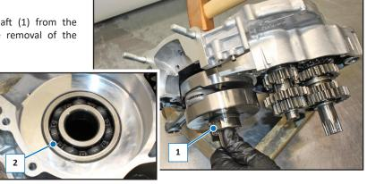
NOTE: Upon reassembly, heat the inside of the bearing (2) of the crankshaft before inserting the crankshaft (1).
