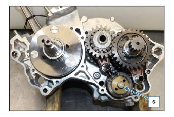
Re-mount the components, proceeding in reverse order to disassembly, lubricating with engine oil and, when re-mounting the gearbox unit, paying attention to correctly position the forks (2, 5 and 7) in the relevant positions:
