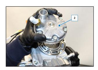
NOTE: Upon reassembly, replace the seals (3) and screw the screws (1) without tightening, then tighten them crosswise with a torque of 20 Nm (2,0 kgm, 14,75 ft/lb).
