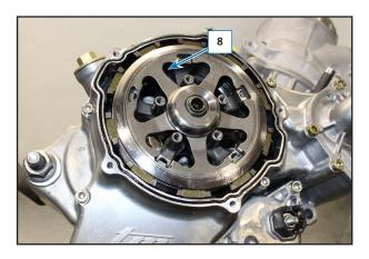
Assemble the cup spring (7) and ring nut (6) inserting the first screw in the hole of the ring nut (6) marked with " • • ", then approach the screws (5) alternatively and tighten them with a torque of 8 Nm (0.8 kgm, 5.9 ft/lb).
