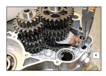
Remove the complete gear assy (2).
