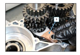
Remove the fork (6) of the secondary shaft.
