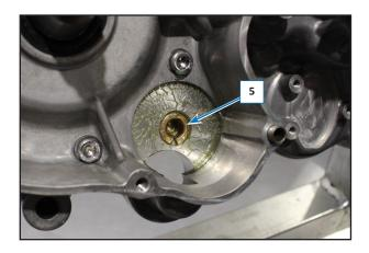
Grease the gears (6) of the Bendix (1) and reassemble it in the bronze bush (5).
