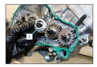
Screw in the flanged nut (1) at a torque of 70 Nm (7 kgm, 51.63 ft/lb).
