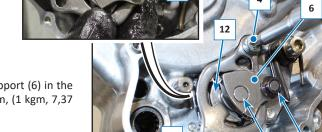
Fit the plate (5) on the pin (11) by inserting the ratchet support (6) in the ring nut (12), tighten the screws (4) with a torque of 10 Nm, (1 kgm, 7.37 ft/lb + Loctite 243).
