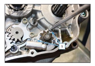
Remove the pump (2) by lifting it.
