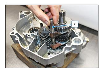
Release the forks (8) and (9) of the secondary shaft from the selector drum and remove them.
