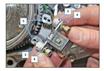
NOTE: On re-mounting, check the distance between the pick-up (2) the reference notch (7) of the flywheel is between 0.7-1.0 mm.
