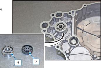
Remove the oil seal (7), operating from the external part of the guard with water pump disassembled.
