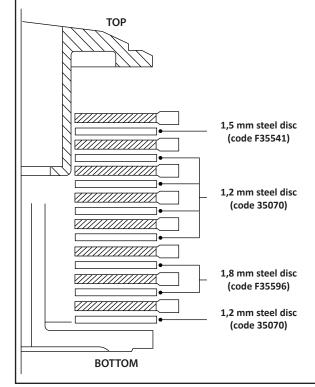
NOTE: When reassembling the new discs, lubricate them with engine oil. Ensure that the first assembled disc is made of steel and 1.2mm thick, then insert the discs as shown in the figure.
