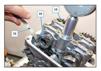
Use a thickness gauge (17) to check the play between the exhaust cams (18) of the intake camshaft (14) and the valve pad is 0.20 mm (0.008 in.).
