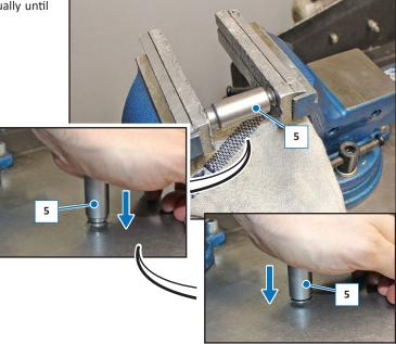
Further press the chain tensioner (5) and release; the mobile part (8) of the chain tensioner (5) must release without obstacles.
