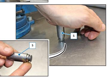
Insert the chain tensioner (5) in the seat of the cylinder.
