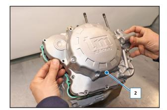
Tighten the screws (1) crosswise, positioning them in the relative housing, depending on their length.
