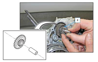
Re-mount the idler (1) with the relative roller bearing cage and lubricating with engine oil.
