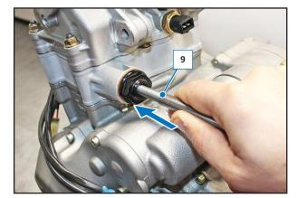
Remount the plug (1) making sure you replaced the OR gasket.
