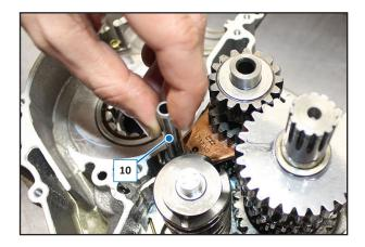
Use a screwdriver to move the ratchet (11), releasing the drum (12), and then remove the drum from the semicase.
