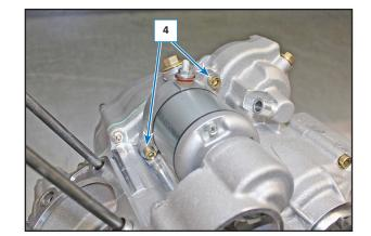
Unscrew the two starter motor fastening screws (4).
