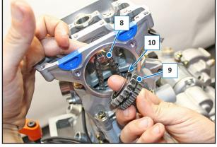
Correctly place the timing chain (8) on the drive gear (9).
