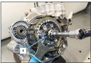
Lock the nut by raising the tabs of the lock washer (2).
