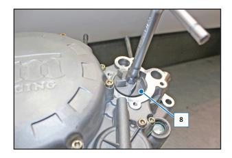
Loosen the pump impeller (8).
