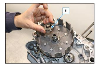
After having re-mounted the bell (6) and the drum (3), make sure the safety washer (2) has been positioned correctly.
