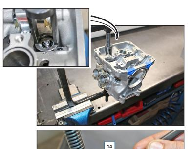
Use a magnet to remove the two half cones (14).
