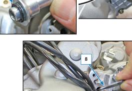
Slide the clutch rod (8) out.
