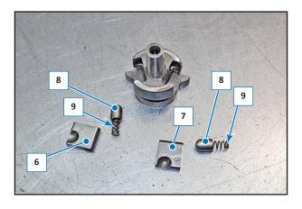
NOTE: On re-mounting, make sure the ratchets (6) and (7) are inserted correctly in the relative housing; they cannot be inverted. Re-mount everything in reverse order to the disassembly operations, checking that the two timing bolts (10), one on the shaft and the other on the ratchet-holder gear, are aligned. Tighten the screw (1) with a torque of 10 Nm (1.0 kgm, 7.37 ft/ lb) and screws (2) with a torque of 10 Nm (1.0 kgm, 7.37 ft/lb) + medium threadlocker (blue).
