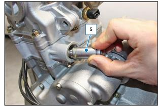
Manually push the chain tensioner (5) so that it inserts correctly on the OR (6) while it enters in its corresponding seat.
