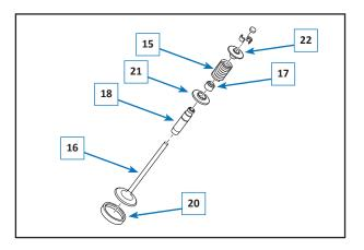
Using the relevant tool, compress the double spring (15) and insert the two half cones (14) onto the valve stem; release the double spring and remove the tool. Check that the half cones (14) are positioned correctly on the stem using a rubber hammer to tap the upper valve stem to position it correctly.
