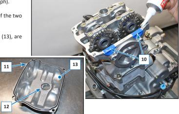
Mount the head cover (13) by screwing the screws (14) crosswise and then tightening them with a torque of 10 Nm (1 kgm, 7.37 ft/lb).
