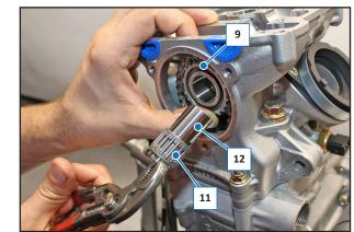
Keep the drive gear (9) in position, lubricate the pin (12) and the bearing (11) with engine oil and mount the drive in its corresponding seat of the head, locking it (9) in position.
