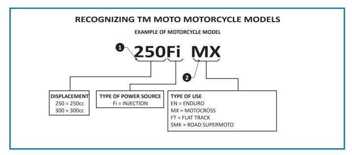
The displacement, type of power source and type of use define the motorcycle model and engine of each TM Racing motorcycle.
