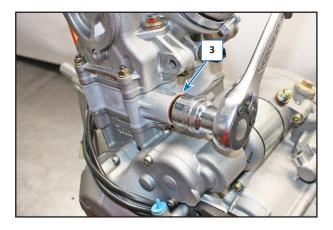
Use a punch (9) to push the chain tensioner so that the mobile part is released while tensioning the chain.
