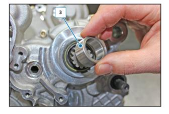
NOTE: When reassembling the bushing (3) replace the "OR" gasket (4). Lubricate the bush (3) and the gasket (4) with engine oil before remounting it.
