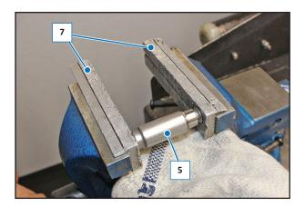
Remove the chain tensioner (5) from the vice and press it manually until end of stroke, checking that it slides without obstacles.
