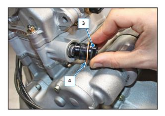
Tighten the plug (3) with a tightening torque of 33 Nm (3,3 kgm, 24,34 ft/ lb).
