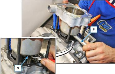
Completely insert the cylinder (2) in the stud bolts (10) by inserting the two sliders.
