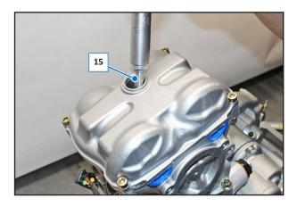
Check the gasket (16), replace it if worn, then remount the plug (17) screwing it with a tightening torque of 20 Nm (2.0 kgm, 14.75 ft/lb).
