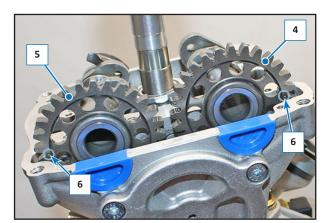
Mount the intake camshaft (4) and the exhaust camshaft (5) so that the tuning points (6) are parallel on the edge of the head.
