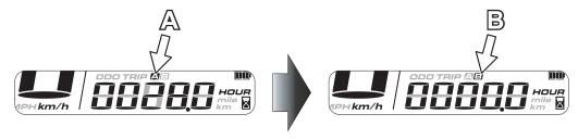
To reset the partial hours of operation both in "A" and in "B" with the function active press the "Adjust" button for three seconds.
