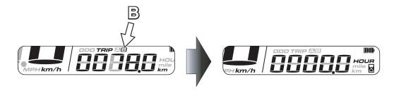
Press the "Adjust" button to switch from the total hours of engine operation to the partial hours of operation "A".
