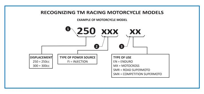
The displacement, type of power source and type of use define the model of motorcycle and engine of each TM Racing bike.
