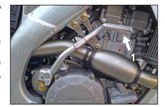
Starting from the highest position, push the starter all the way down with fast, continuous movements.
