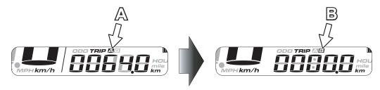
To reset the km/miles travelled both in "Trip A" and in "Trip B" with the function active press the "Adjust" button for three seconds
